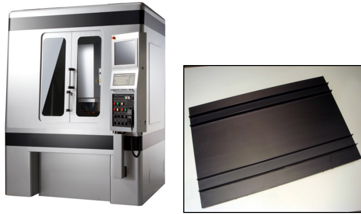
(a) CFRP X-Y table mounted on a machine tool (Sodick Co., Ltd.)
